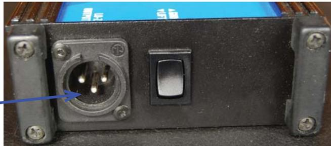
Figure I-8 Connecting XLR to Direct Box
